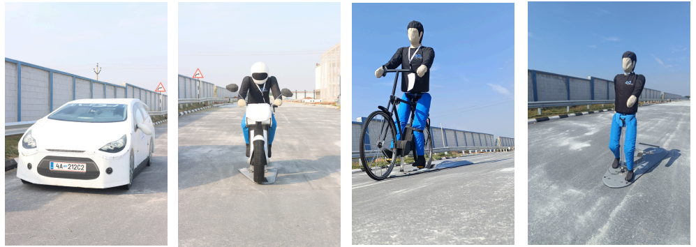
EuroNCAP Certified Soft Targets for Active Safety
